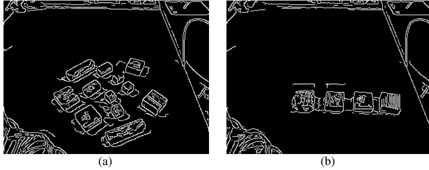
Fig. 5. Canny edge detector applied to the original images.
